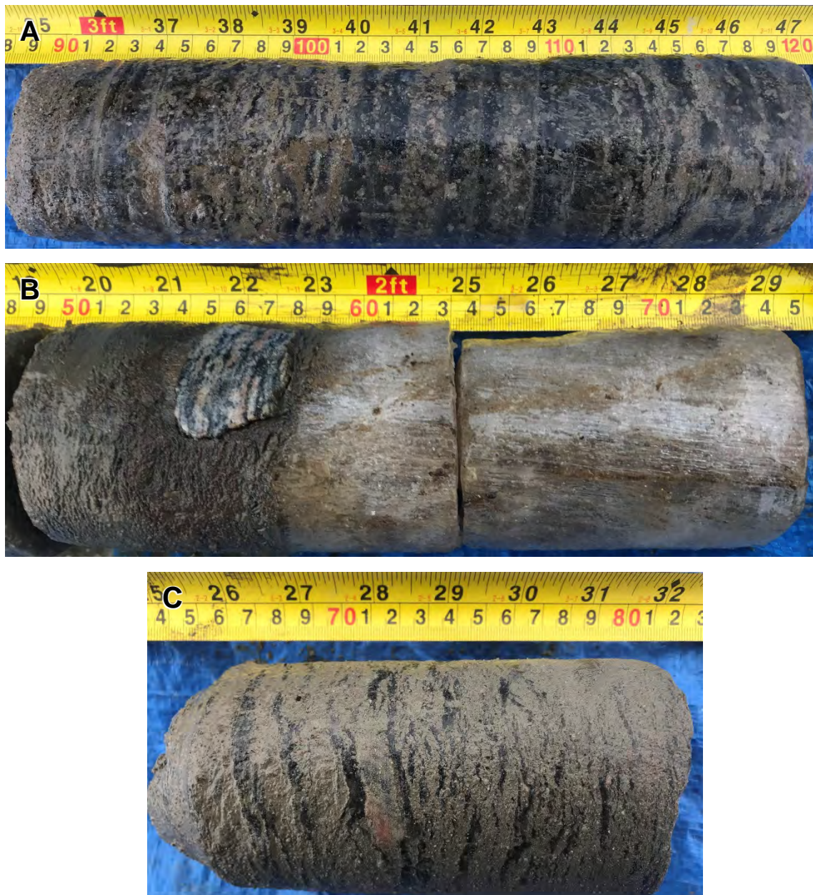
Figure 4-3 Examples of ice-rich permafrost core samples.
