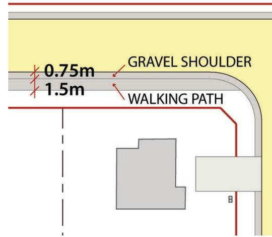
Figure 28: Dedicated walking paths located within road rights-of-way should be at least 1.5 metres wide, plus the width of the gravel shoulder, for a total of 2.25 metres. Vertical barriers (e.g. bollards or boulders) can be placed in the shoulder to protect pedestrians from vehicle traffic.
