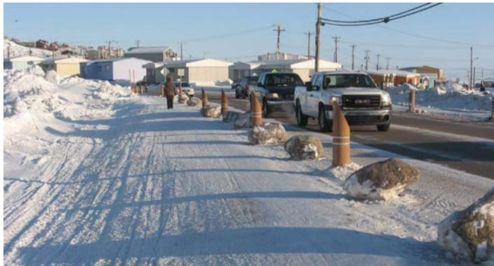
Figure 29: Pathways can be located within road rights-of-way. Elements such as bollards and boulders have been used to separate the pathway from vehicle lanes.
