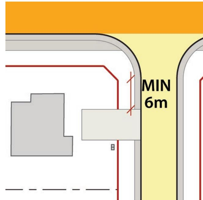
Figure 34: Driveways should be located a minimum of 6 metres from intersections and turning radii.
