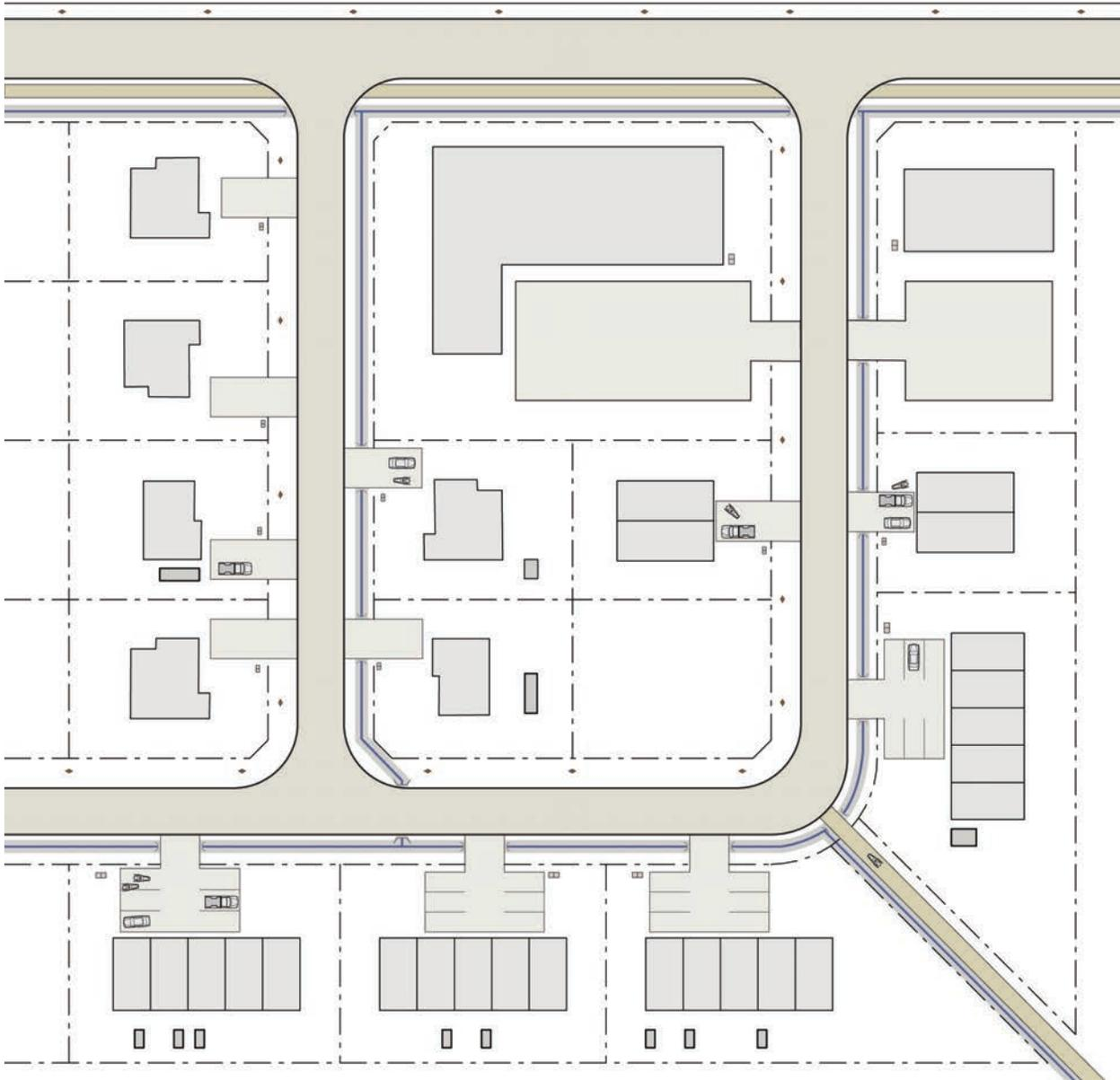
*Figure 38: Ditches and culverts should be located within road rights-of-way and be properly maintained to avoid flooding and stagnant pools of water.*
