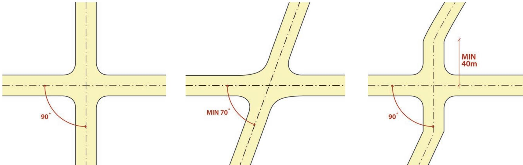
Figure 32: Roads meeting at an intersection should ideally meet at perpendicular angles (i.e. 90°). The minimum angle of intersection is 70° in cases where a perpendicular intersection is not possible. One solution to a road intersecting another at an angle is to straighten the angled portion to 90° at least 40 metres from the centre of the intersection.
