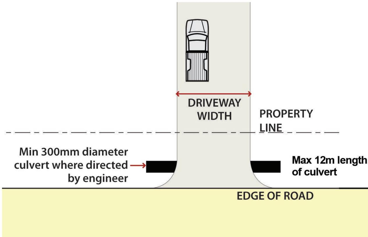
Figure 39: Culverts should be installed under driveways in line with any ditches in the road right-of-way according to engineering specifications.
