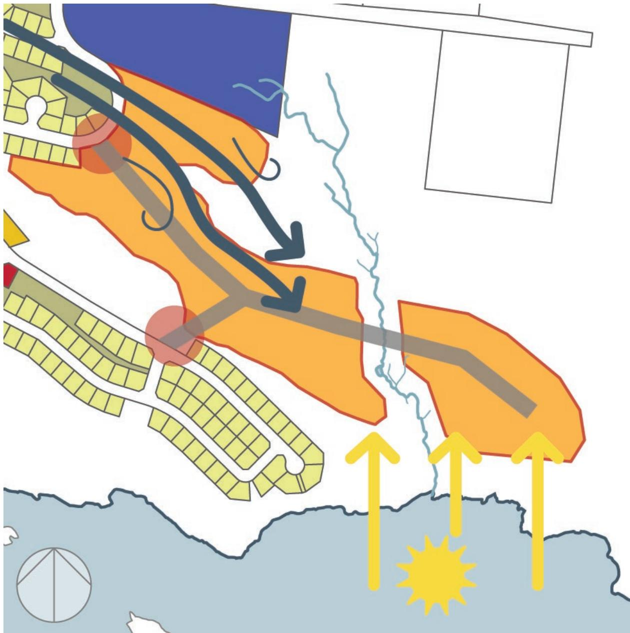
Figure 21: To determine a conceptual road layout, consideration must be given to prevailing wind direction (blue arrows) solar orientation (yellow arrows), and road access points (red dots) to the development area. The optimum conceptual road layout will need to balance these guidelines in addition to consideration for drainage.
