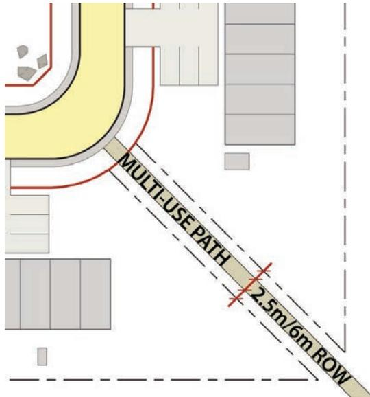
Figure 35: Multi-use trails (e.g. pedestrian, snow machine, ATV) should be a minimum of 2.5 metres in width and be located within a minimum 6.0 metre right-of-way. Drainage ditches can be incorporated into the rights-of-way for multi-use trails; however the right-of-way may need to be widened.
