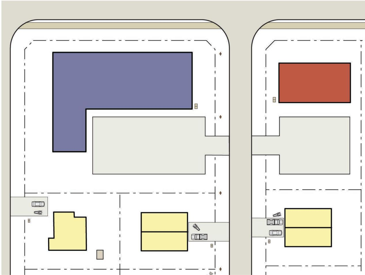
*Figure 45: Major commercial uses (red building) and community uses (blue building) should face collector roads and preferably have vehicle parking located in the side and rear yards.*
