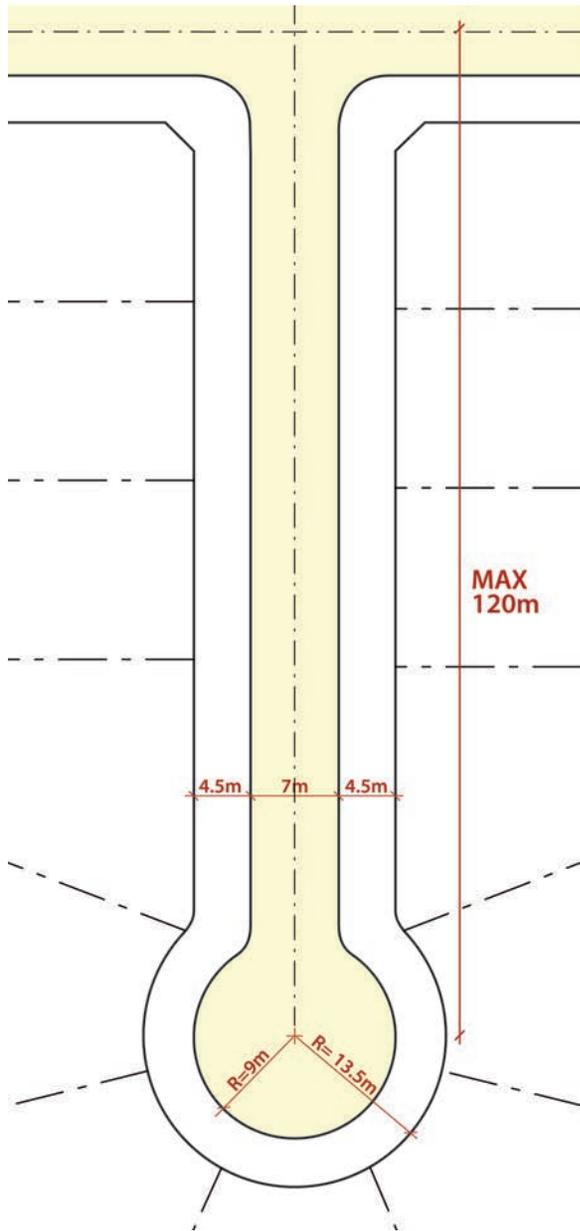
Figure 33: Cul-de-sacs on local roads should have a minimum right-of-way radius of 13.5 metres and a minimum road surface radius of 9 metres. The maximum length of a road ending in a cul-de-sac is 120 metres.
