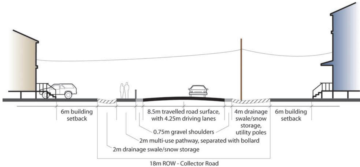
Figure 25: Collector road rights of way on trucked service should be at least 18 metres wide to allow for road lanes, shoulders, pedestrian walkways, drainage ditches and utility poles.
