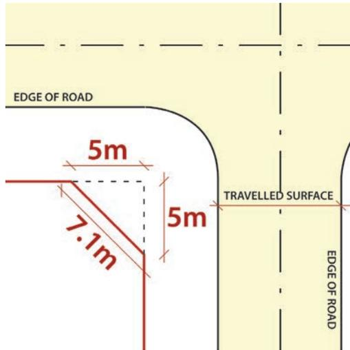
Figure 31: A “splay” of at least 5m in length must be incorporated for corner lots.
