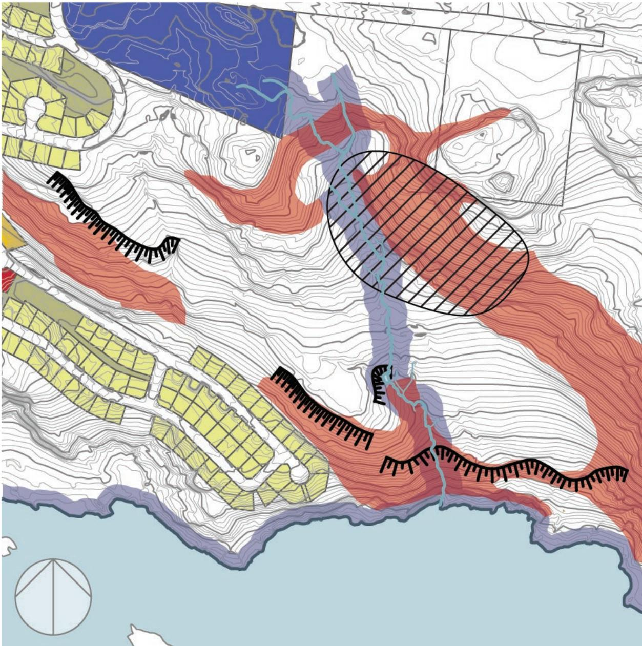
Figure 18: Site analysis responds to guidelines by identifying steep slopes greater than 15% (red), water body setbacks (light blue), snow drifting areas (black hatching), and significant rock outcrops (black).
