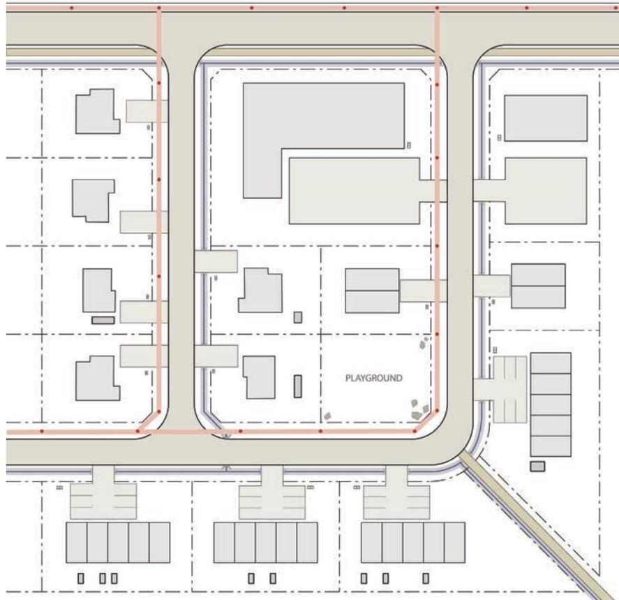
Figure 48: Power poles and power lines should be contained within the road right of way, typically on the opposite side from any drainage ditches and designated pedestrian walkways.
