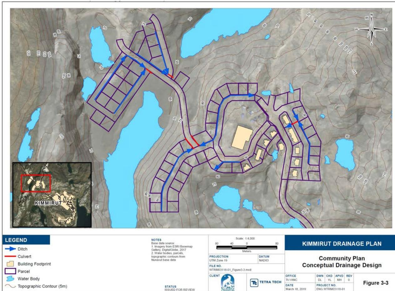
Figure 12: A conceptual design of a drainage master plan for a subdivision in Kimmirut
