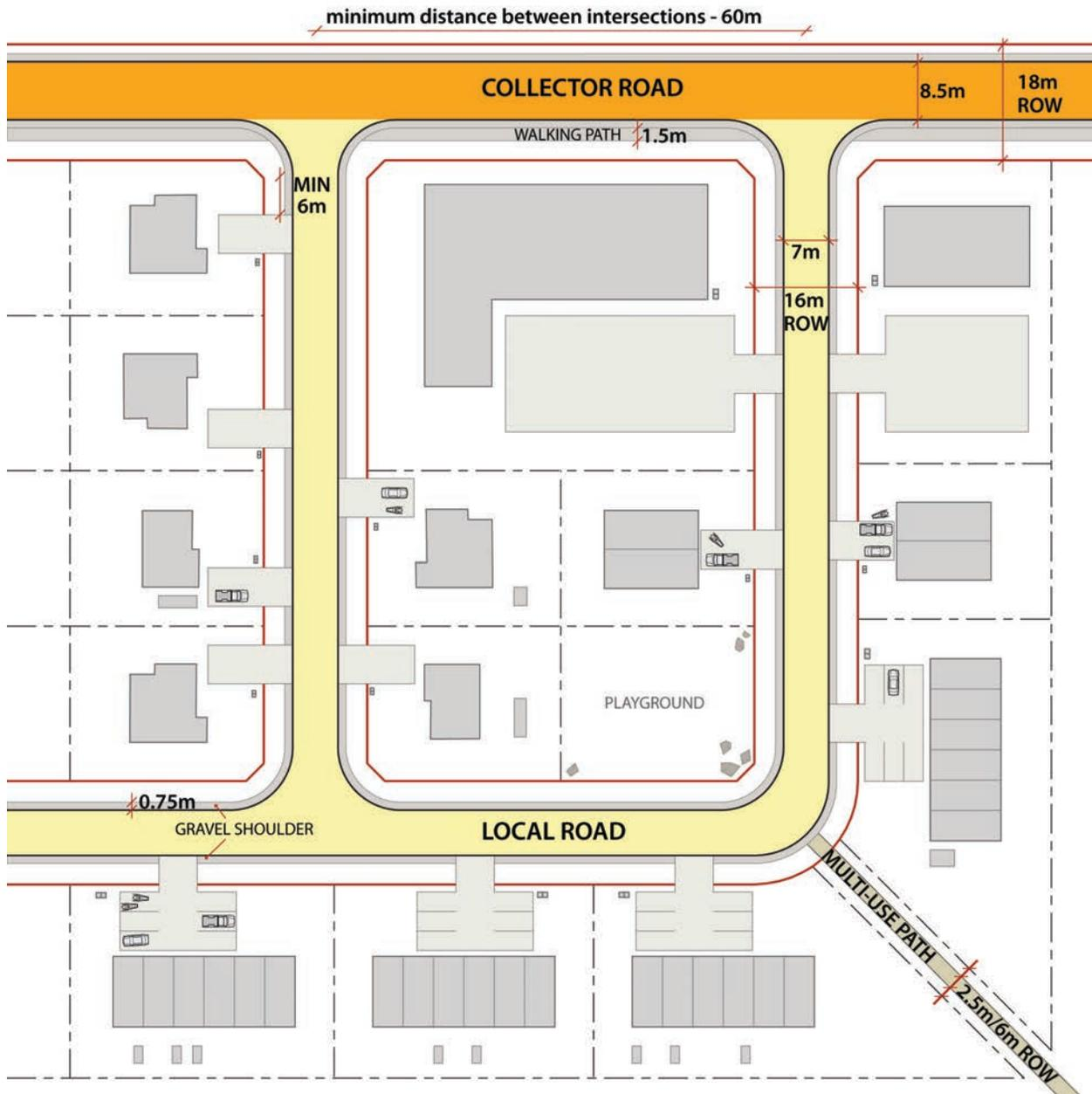
Figure 24: Minimum widths for the rights of way and the traveled road surfaces are illustrated for collector (orange) and local (yellow) roads within a subdivision on trucked services.
