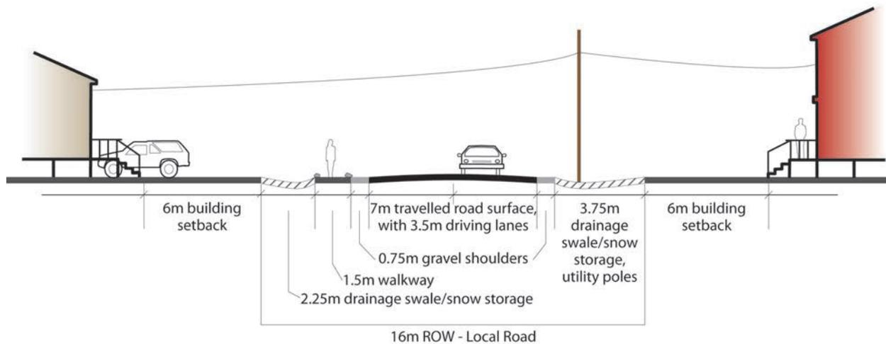
Figure 26: Local road (two-way) rights of way on trucked service should be at least 16 metres wide to accommodate road lanes, shoulders drainage ditches and utility poles
