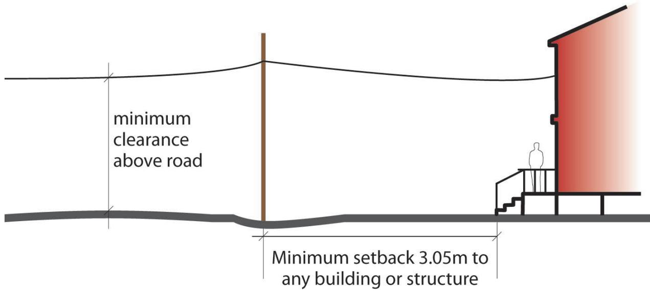
*Figure 52: Power poles and power lines must be setback from buildings and structure and must provide for minimum clearance above roads and other travelled surfaces.*
