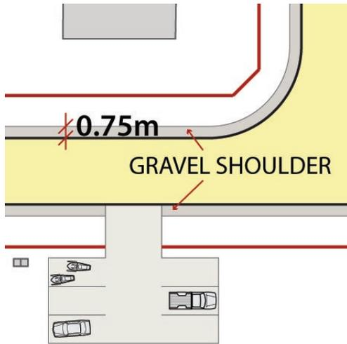
Figure 27: Gravel shoulders of at least 0.75 metres width should be incorporated into all local and collector road designs.
