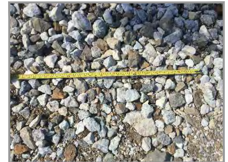
TYPICAL 50-75 mm (2-3") CLEAR CRUSH GRADATION SCALE:NTS
