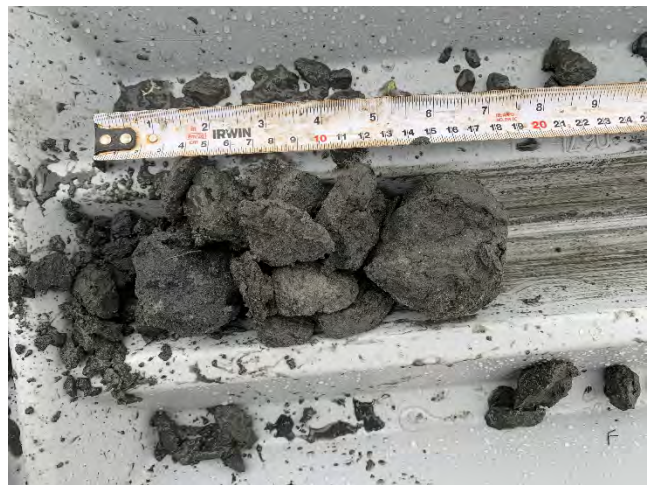
Photo 28: Photo of moderate ice content permafrost recovered at Borehole BH21-01. Includes well-bonded cryostructures with excess ice (Nbe).
